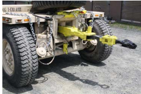
TeleSwivel™ Hitch on M989A1 (with Lift Assist Kit)
