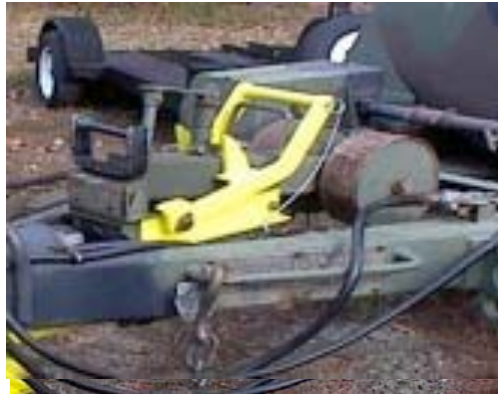
Landing Leg Assist Kit (secured)
